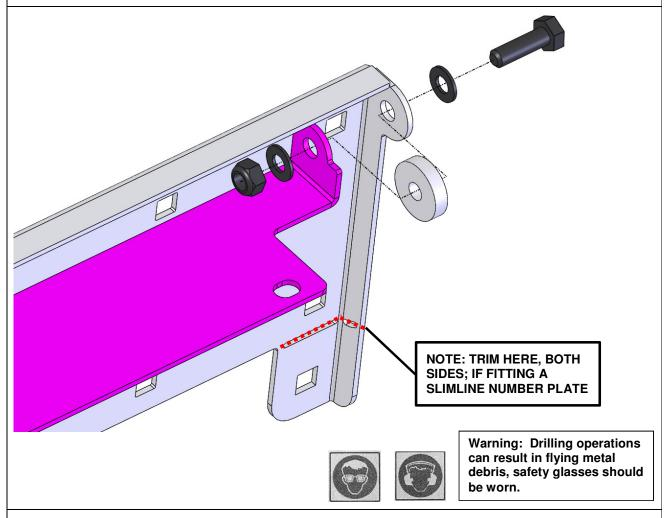
42. Assemble the bracket assembly to the bar using the fasteners supplied with the bar fitting kit. Follow the step in the bars fitting instructions showing the fixed license plate bracket being mounted substituting the folding assembly for the fixed.
