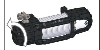
**Bushranger winches**: Undo the screws in the gearbox end of the winch to remove the brake cover. Remove the bolts retaining the gearbox housing.
