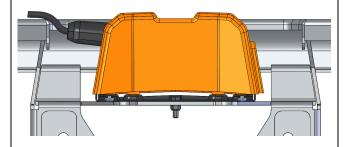
**HINT:** Apply some split cable protection conduit to the winch cables where they pass through the Bull Bar then route and cable tie them clear of the winch spool.
