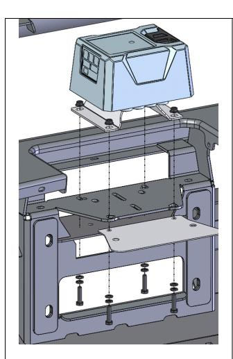
17. Adjust the control box until it is approximately 5mm clear of front of control box recess and tighten all fasteners.
