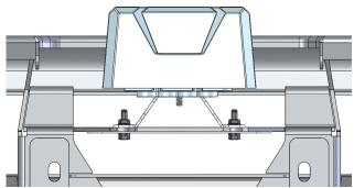
**HINT:** Apply some split cable protection conduit to the winch cables where they pass through the Bull Bar then route and cable tie them clear of the winch spool.
