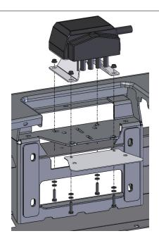
21. Adjust the control box until it is approximately 5mm clear of front of control box recess and tighten all fasteners.
