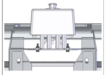
**HINT:** Apply some split cable protection conduit to the winch cables where they pass through the Bull Bar then route and cable tie them clear of the winch spool.
