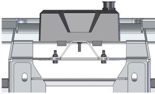
**HINT:** Apply some split cable protection conduit to the winch cables where they pass through the Bull Bar then route and cable tie them clear of the winch spool.
