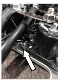
7. Undo 2x supplied M6 nuts from underside of control box. To do so, top of M6 bolts located on the inner side of the box will need to be held in place.
