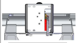
**HINT:** Apply some split cable protection conduit to the winch cables where they pass through the Bull Bar then route and cable tie them clear of the winch spool.
