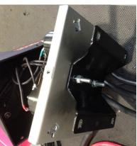
8. Attach control box to control box bracket using fasteners removed from control box in earlier step, so that the top face of the bracket is flush with the bottom surface of the control box.
