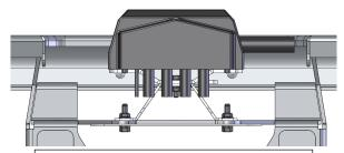
**HINT:** Apply some split cable protection conduit to the winch cables where they pass through the Bull Bar then route and cable tie them clear of the winch spool.
